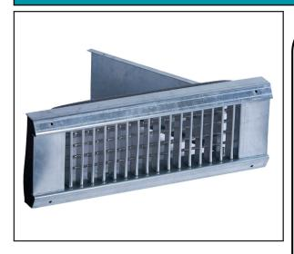
The DMR is a supply/return register with adjustable double deflection blades and a volume damper designed specifically for direct mounting on a spiral duct. The use of rectangular register taps are not required.
